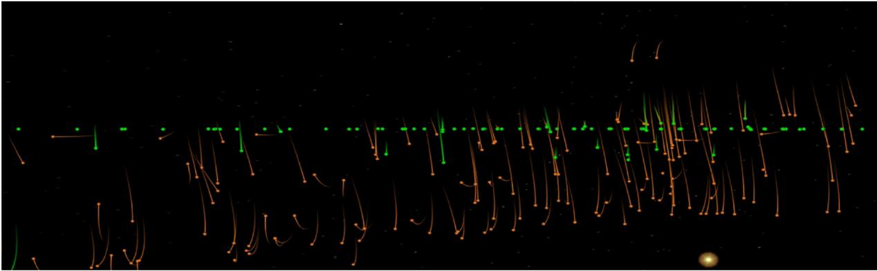
Fig. 7. Typical active GEO satellite-vs-inclined debris approach paths as viewed from within the equatorial plane looking radially outward. Green dots are active GEO satellites and orange dots are current GEO debris. (For interpretation of the references to colour in this figure legend, the reader is referred to the Web version of this article.)
