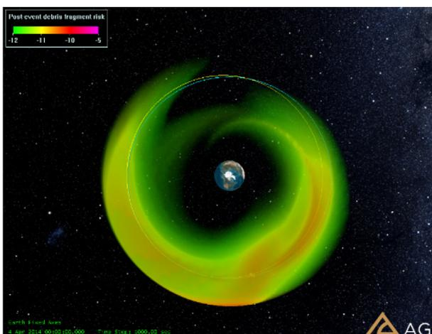
Fig. 72. Total fragmentation risk in the Earth-fixed frame, aggregated over a 28 h analysis timespan.
