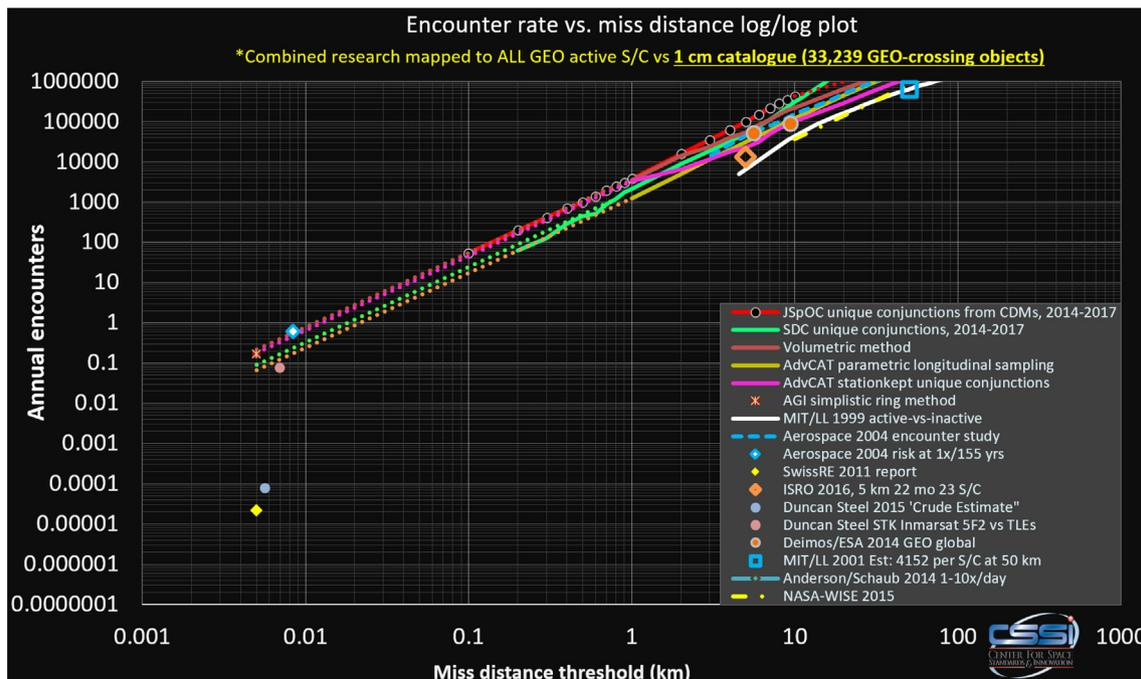
Fig. 67. Scaling of GEO encounter rates to all active GEO satellites vs 33,239 estimated satellites and debris > 1 cm.
