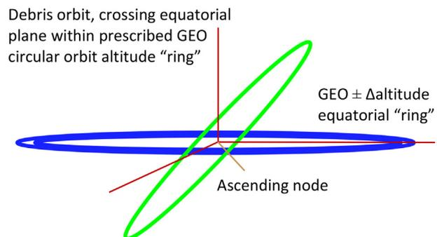
Fig. 58. “Ring” method determines collision likelihood from all catalogue orbits crossing an equatorial GEO ± 10 km planar ring.
