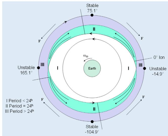
Fig. 51. Gravity well positions for GEO debris.
