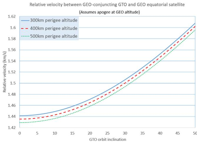
Fig. 24. Relative velocity between GEO equatorial satellite and GEO-conjuncting GTOs with 300, 400 and 500 km perigee altitudes.
