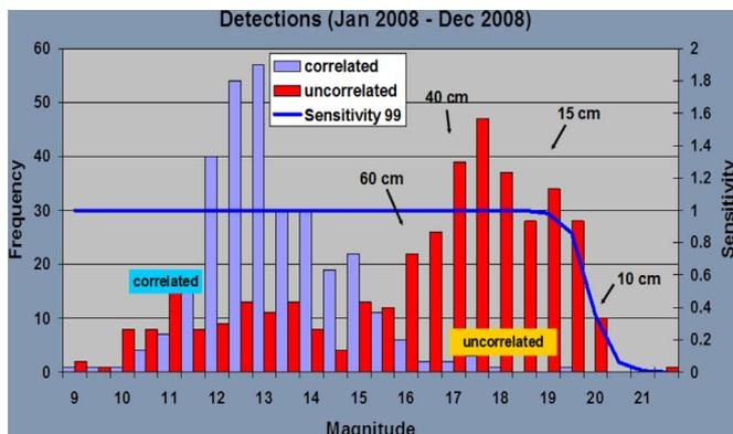
Fig. 2. GEO object detections obtained in ESA’s optical sensor debris campaign (2008) [15] (included by permission of author).
