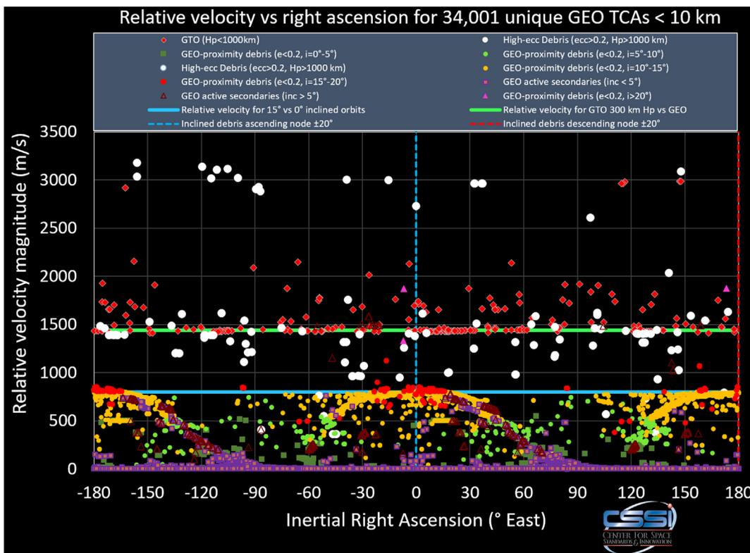
Fig. 16. Detailed forensics of relative velocities for 34,009 JSpOC close encounters by secondary (conjoining) object orbit type.
