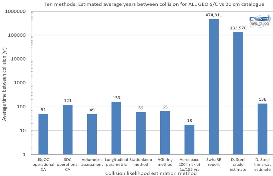
Fig. 66. Average years between collisions for all active GEO satellites vs 1912 estimated satellites and debris > 20 cm.
