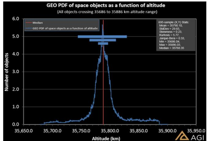
Fig. 39. Longitudinally-averaged Probability Density Function of GEO satellites and debris as  $f$ (altitude).
