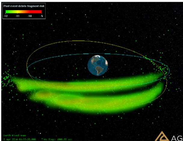
Fig. 71. Estimated fragmentation cloud dispersion volume at 15 h after collision (Earth-fixed frame).
