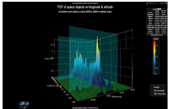
Fig. 38. Probability Density Function of GEO satellites and debris as a function of longitude and altitude.
