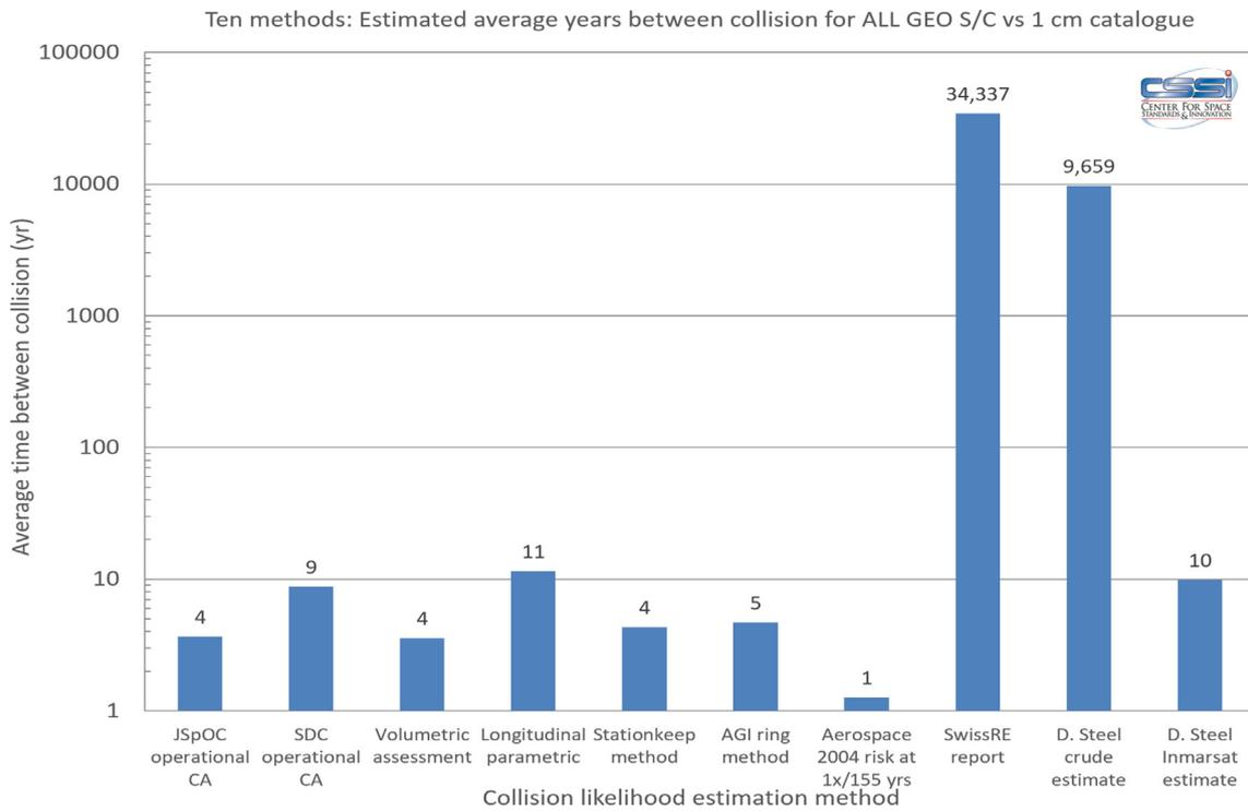
Fig. 68. Average years between collisions for all active GEO satellites vs 33,239 estimated satellites and debris > 1 cm.
