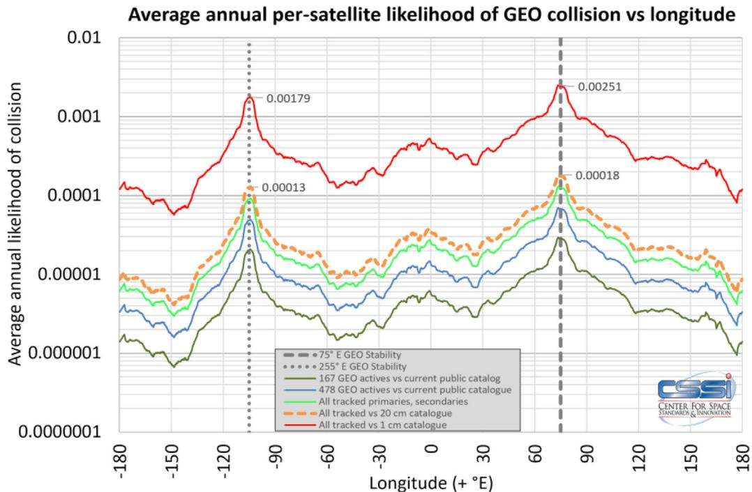
Fig. 69. Per-satellite likelihood of GEO collision by active/debris category and by longitude.
