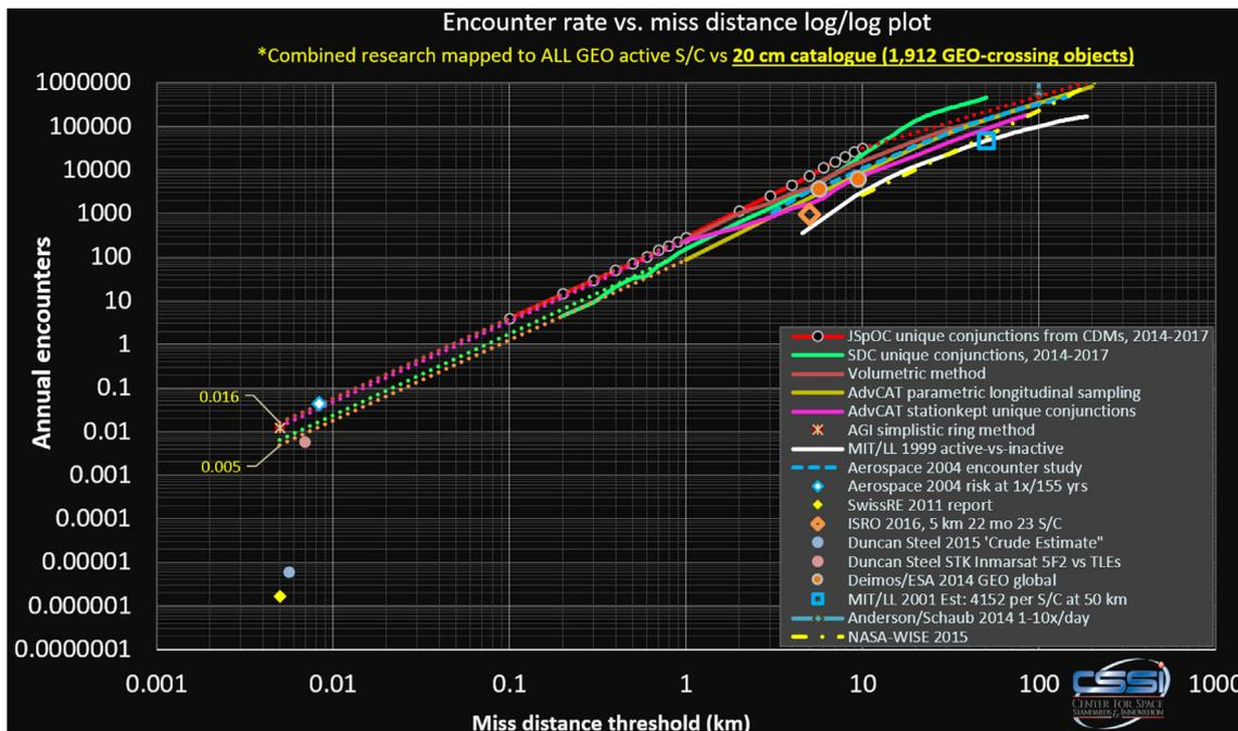
Fig. 65. Scaling of GEO encounter rates to all active GEO satellites vs 1912 estimated satellites and debris > 20 cm.
