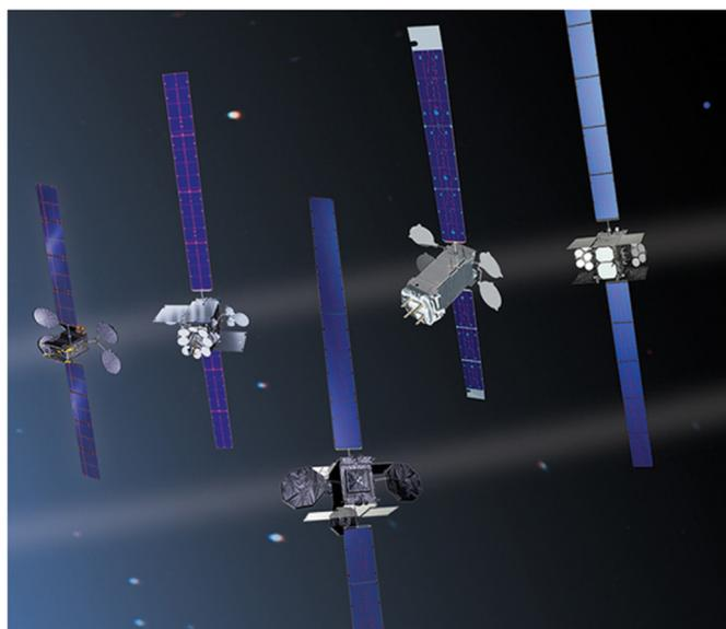
Fig. 5. Boeing 702 satellites flying in their typical GEO satellite orientation, with long dimension aligned north/south to allow the solar arrays to track Sun.
