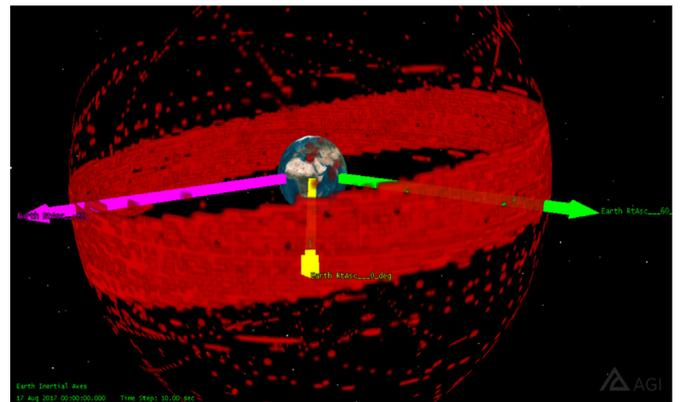
Fig. 19. Equivalent 3D spatial density volumetric of all GEO ± 100 km altitude-crossing objects, including vector aligned with Vernal Equinox (yellow) and two vectors in equatorial plane 60° away. (For interpretation of the references to colour in this figure legend, the reader is referred to the Web version of this article.)
